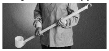
For easy sampling from tanks, vats, lakes, etc., these high-density polyethylene dippers will not rust or corrode and provide excellent chemical resistance. 29mm (1 1/8") diameter handle is welded to the rigid bowl at a 45 degree angle. The 3.7M (12 ft) handle is available in one piece or two-piece screw-together construction. The end of the handle has a hook for hanging. Orders may be customized by substituting scoops in place of cups. Other styles made to order. 12 per case.
