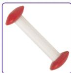
**Circulus™** magnetic stirring bars provide strong turbulence at relatively low speeds, offer reduced surface contact and have excellent centering characteristics, particularly in vessels with convex bottoms.
