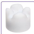
**Cell** magnetic stirring bars are designed specifically for use with spectrophotometer cells, cuvettes or test tubes. The cell stirrer fits into standard 10mm spectral cells and provides rapid vertical and horizontal mixing with a minimum of vortexing when placed on a magnetic stirring machine. Centrifugal pumping action, generated by the cross channels in the upper face, mixes without aeration.
