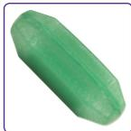
**Fluted Octagonal - Rare Earth magnet** The flutes of this eight-sided bar along with a definitive tapering to conical ends provides excellent surface area and recessed breaks in the profile to generate strong turbulence and efficiently move fluids. Available only in Rare Earth (Samarium Cobalt), the shape and magnet strength make these bars especially well-suited for viscous solutions.
