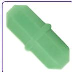
**Octagon - Rare Earth magnet** The superior magnetic energy of Rare Earth (Samarium Cobalt) magnets provides strong coupling with drive magnets reducing frequency of spinout in viscous solutions or high speed stirring. The bright green Teflon® PTFE coating makes them easy to identify in the laboratory.
