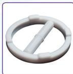
**Spinring®** stirring bars provide maximum stabilization of the magnetic stirring bar with the addition of a "hoop" around a standard octagonal bar. The friction fit of the "hoop" and bar allows them to spin as a unit. By presenting a greater surface area and wider profile, "spin out" is virtually eliminated. This particular arrangement is best suited for larger open-neck vessels, such as buckets and beakers.
