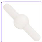
**Saturn Spinbar® Magnetic Stirring Bars** easily stir powders into solutions without getting stalled. A prominent sphere in the middle of the bar elevates the stirring bar arms during rotation and consequently diminishes the surface contact area, permitting the magnet to spin freely without stalling. For use in round or flat bottom vessels.
