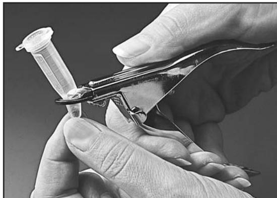
**NOTE:** Insert the new blade with the concave, crescent-shaped cutting edge facing down (away from the fixed blade).
