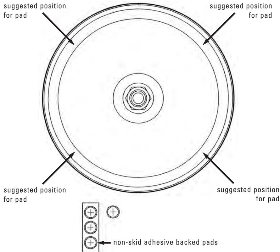
1. Apply the four (4) non-skid adhesive backed pads, included with your Scienceware® Weighted Base Bracket, to the four positions on the underside of the base.
