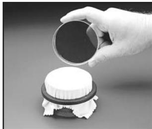
Mark a spot as a circumference reference point on the locking ring (correction fluid provides a convenient, quick-drying mark) for the master plate and all subsequent replica plates. This allows for alignment of colonies. Place the PVC round block on a laboratory bench, large end down. A single velveteen square is centered and placed face-up on the flat top surface of the block.
