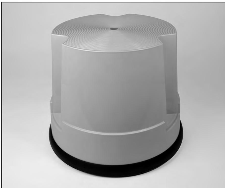
The Safety Step Stool features a wrap-around rubber bottom skirt that gives a non-skid contact with the floor. The stool rolls on three spring-loaded swiveling casters. When weight is placed on the stool, the casters recede against compression springs and the stool will rest directly on the floor. When weight is removed, the springs push the casters out for easy rolling on the floor. The stool rolls easily on any smooth hard surface and will also roll well on low-pile carpets.
