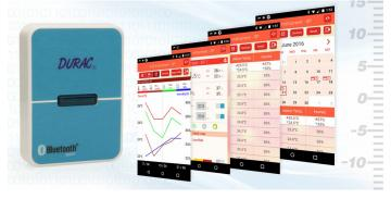
Hourly data is recorded for up to seven days, then maximum and minimum temperatures (model B60911-0100) or temperature and humidity data (model B61506-5100) are recorded for the next 23 days. An alarm will sound if the temperature falls outside of the set parameters.
