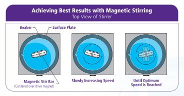
Vertical distance between the drive magnet and the stirring bar should be kept to a minimum for the best coupling and stirring efficiency. Therefore, the containing vessel should be as thin as practical.
