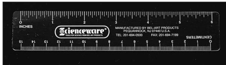
The Fluorescent ruler can be in observing and photographing Ethidium Bromide stained nucleic acid agarose and acrylamide gels. The scale will fluoresce visibly upon illumination with ultraviolet light. This serves as a measure of nucleic acid mobility, and can be used to quantify the sizes of the nucleic acid fragments. This measurement will also allow the comparison of gels run at different times under the same conditions.
