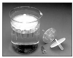
maintains a constant pressure on the tube caps protecting them from opening under internal air expansion. A <sup>3</sup>/16" (4.8mm) thick polypropylene disk is centrally mounted on a threaded handle. The racks float while 1.5ml microcentrifuge tubes remain immersed at a constant depth regardless of water level. The TPX
