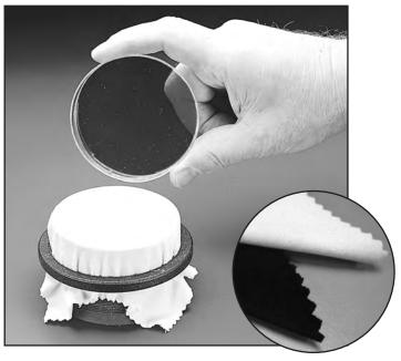
These 100% cotton, sterile Velveteen Replica Plating Squares are especially suited for use in conjunction with the Scienceware® Replica Plating Tool #F37848-0000.
