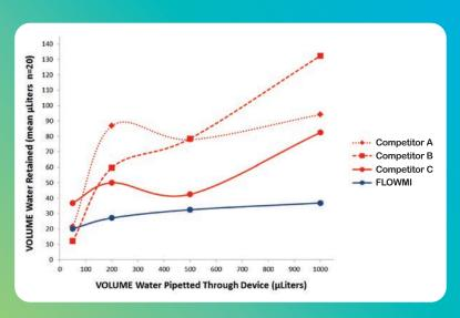
FLOWMI™ and three competing strainers were examined at four pipetted volumes (50, 200, 500, and 1000 µl). The Volume of Water Retained (µl) by each strainer, at each pipetted volume, is represented by the mean difference in weight before and after pipetting water through the strainer. (n=20 per pipetted volume; each trial using a new strainer).
