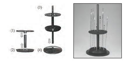
Using the photograph as a guide, press the disc with concentric grooves onto one end of the short larger diameter tube, then press the disc with multiple holes onto the other end of the short, large diameter tube. Make sure these three parts are firmly pressed together
