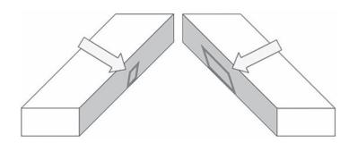
2. When building your rack system you should position the first rack with the smaller 'side lock' in the direction you intend to build. This way as you add racks you can easily lower the larger side lock onto the smaller side lock and the 2 units will simple lock into place.
