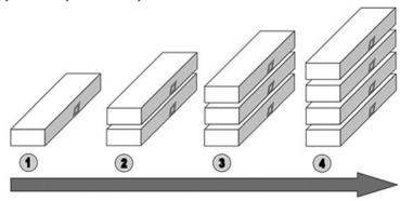
5. If you are building your rack system in a Right-to-Left direction, simply start out with your Scienceware Ultra Low Freezer Wire Rack with the smaller 'side lock' facing out. Since the Front and Back of the Scienceware Ultra Low Freezer Wire Racks are the same, equal assembly ease is available to you regardless of the direction you decide to build your rack system from.
