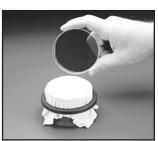
Mark a spot as a circumference reference point on the locking ring (correction fluid provides a convenient, quick-drying mark) for the master plate and all subsequent replica plates. This allows for alignment of colonies. Place the PVC round block on a laboratory bench, large end down. A single velveteen square is centered and placed face-up on the flat top surface of the block.
