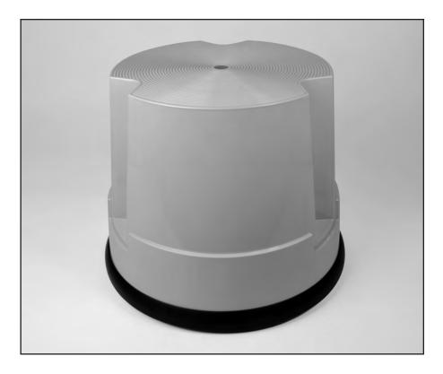
The Safety Step Stool features a wrap-around rubber bottom skirt that gives a non-skid contact with the floor. The stool rolls on three spring-loaded swiveling casters. When weight is placed on the stool, the casters recede against compression springs and the stool will rest directly on the floor. When weight is removed, the springs push the casters out for easy rolling on the floor. The stool rolls easily on any smooth hard surface and will also roll well on low-pile carpets.
